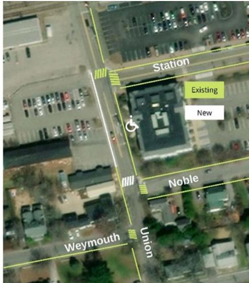
\$100,000 to install a 185 foot long asphalt sidewalk on the west side of Union Street from the Gorham Bike & Ski building to the north side of Station Avenue.
