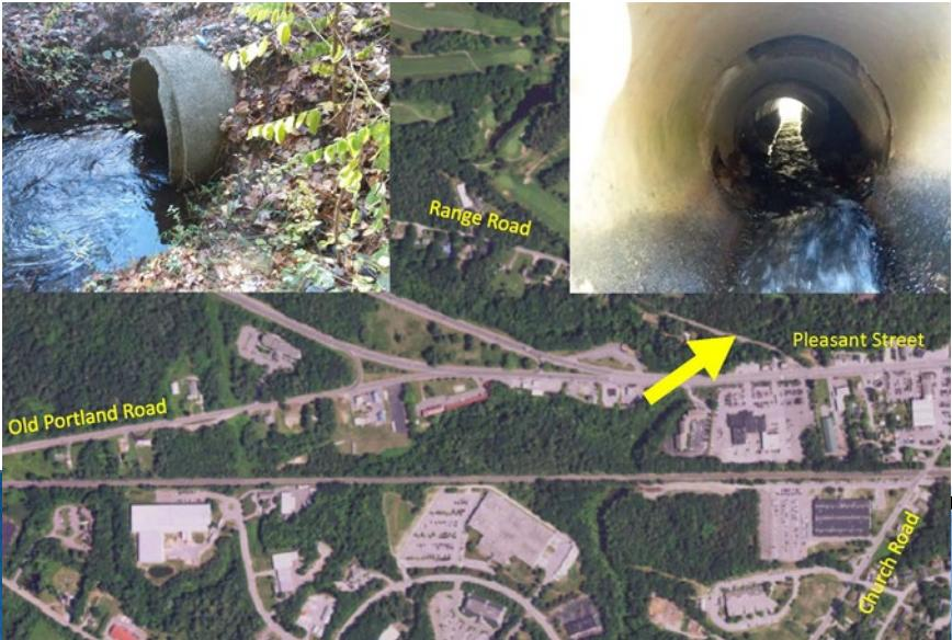
\$20,000 to design and permit the replacement of a 60 linear foot, 42 inch diameter reinforced concrete culvert that crosses Range Road about 400 feet in from Pleasant Street.
