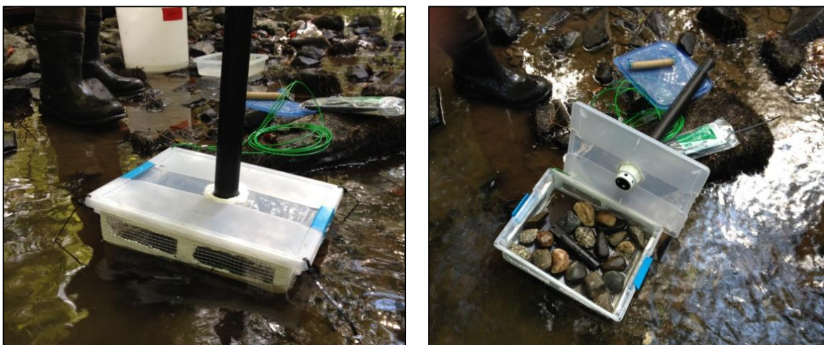
Figure 1. In-stream chambers used to standardize physical habitat conditions between sites. The chambers are filled with cobble-sized rocks to provide suitable macroinvertebrate habitat. They have mesh openings on all sides to allow water to flow through the enclosure. The black pipe on the top of the chamber allows access for a water quality probe to monitor conditions inside the enclosure.
