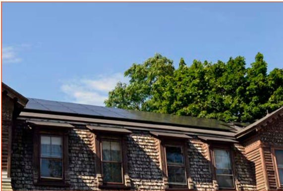
Low profile solar panels minimize the visual impact on the character of a building.
