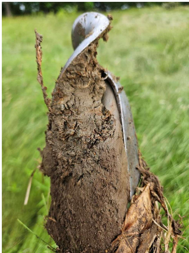
Photo 3: Hydric, mineral soil from a Lacustrine sediment deposit in the wet meadow. Iron concentrations in the gray soil layer near the surface is indicative of a hydric soil.
