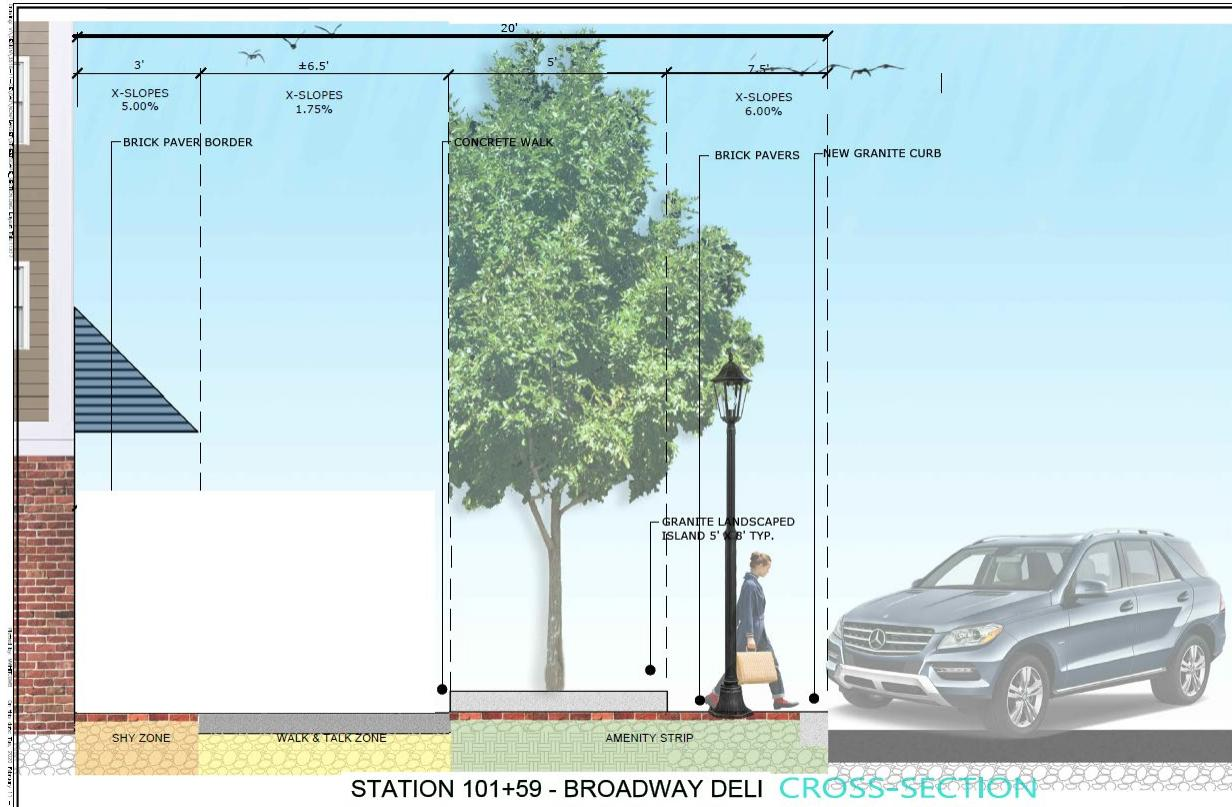
Original Design – Note only about 9 ft of space between building face and tree well/slopes back to existing grade, 5 ft of which must be reserved for ADA use. Also note high slopes next to building face and curb line.
