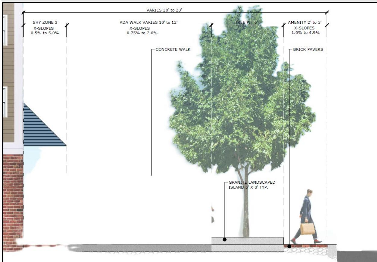
New Design – Note about 15 ft of space between building face and tree/well slopes back to existing grade. This more than doubles the outdoor space for possible business use, while also flattening the grades along the building face and curb line.
