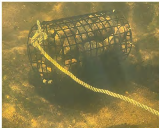
Figure 4-1: Rock Baskets Deployed at Sampling Location Downstream of Brunswick Dam, July 28 2025
